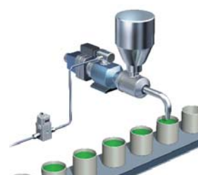
Discharge rate control
